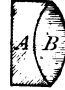
FIG. 57.—Achromatic lens. A, Plano-concave lens of flint-glass; B, biconvex lens of crown-glass.
